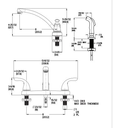
Ø1-3/8 Min to Ø1-1/2 Max. Deck Hole Openings
